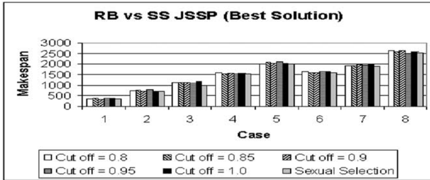
Figure 34. Best Results obtained by Rank-based Selection compared against Sexual Selection (population = 30, generation = 300).
