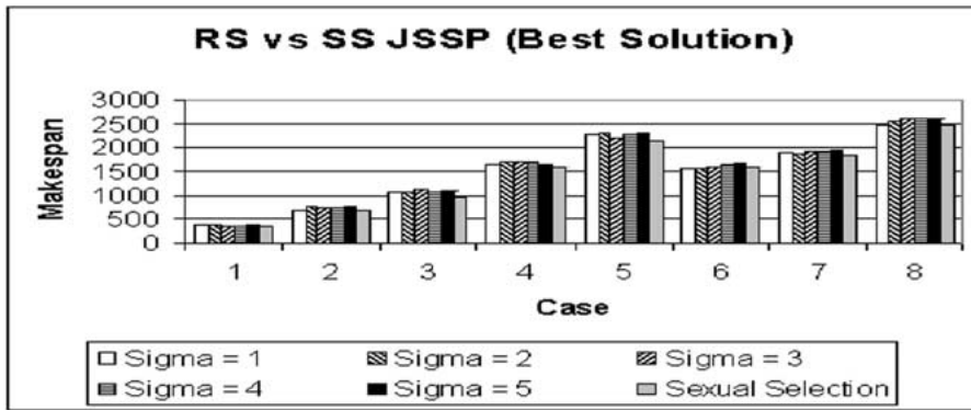
Figure 36. Best Results obtained by Roulette Selection compared against Sexual Selection (population = 50, generation = 500).
